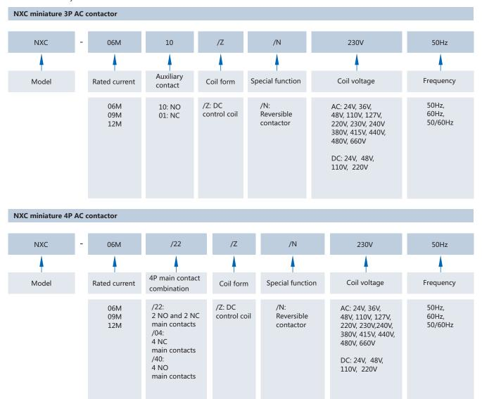
Model example: NXC-12 240V 50Hz represents an AC contactor under AC-3 utilization category that provides a rated current of 12A at a main circuit voltage of 380V/400V/415V. Each contactor body contains one NO auxiliary contact and one NC auxiliary contact. The coil control voltage and frequency are 240V AC and 50Hz respectively.
