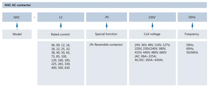
Note: 06A-100A products contain one NO auxiliary contact and one NC auxiliary contact. 120A-630A products contain two NO auxiliary contacts and two NC auxiliary contacts.
